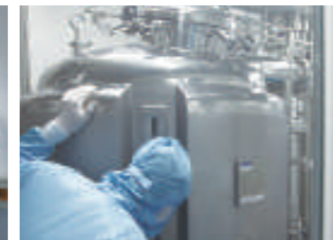
Fully automatic dosing system Batch output 1000 L
