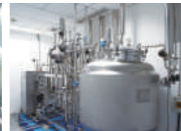
Distilled water system Ensure endotoxin below 0.015 EU/ml
